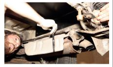
the bolts home from outside in. This powder coated bracket is the key to M1 in-Van approval and provides loads of extra strength to this part of the floor.
