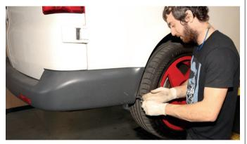
Then undo the T20 / T25 Torx screws (two visible in the back 'arches / two underneath the 'arch liners)
