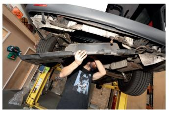
Pop the plastic undertrays back into place and secure with all of the 10mm bolts and new lock washers throughout. Don't forget to replace your spare wheel and hanger as well
