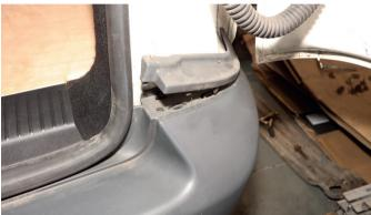
You need to remove your rear bumper so start by popping off the top trim pieces inside the doors, removing the plastic screw-in trim clips with an Allen key (two up top, three beneath the Van)
