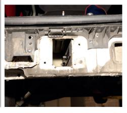
Insert the captive nut plates that slide into the chassis rails. If your Van has a tow bar attachment in here, you can still use the Rusty Lee fitting kit, just without these plates
