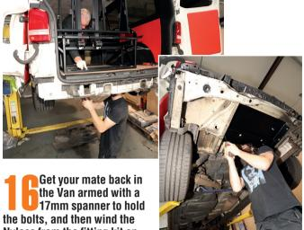
Nylocs from the fitting kit on tight from beneath the Van
