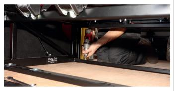
For added piece of mind, and to ensure the bed sat perfectly level, two further holes were drilled through the front rail of the bed. The one closest to the wheelarch fell 170mm from the 'arch, in a double-skinned section just between the spring and chassis rail underneath, so you may have to drill at a slight angle here. Measure twice and drill once
