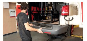
Then slide your rear bumper back on, ensuring the pegs line up with the front mounts in the 'arch liners. Replace all of the Torx screws you took out earlier
