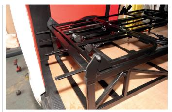
Measure 260mm in from the rear step cover and position the lower back stay of the seat accordingly. Have a friend hold the seat in position and try to extend it fully into a bed, ensuring it clears both side panels freely. If you've used 6mm ply panels or backing foam, your trim could protrude further out so it's worth checking now. Our frame was positioned 50mm square from the wheelarch to clear a crossmember beneath
