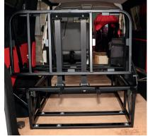
Alian the bed over the holes and drop all six M10 bolts through using the supplied spreader plates on top
